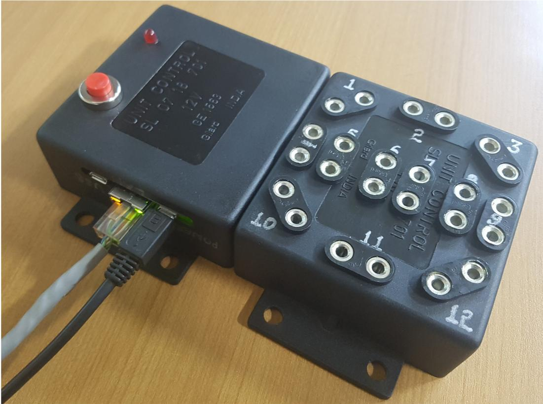
The PCMD-12P is a interface device to link your process to GAP-OSM.
